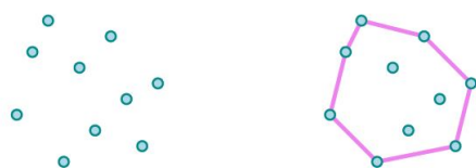
Figure 1 Left: the set P of 10 points in the plane. Right: the convex hull of P .
