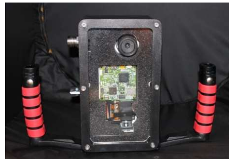
“Hippo” (For underwater structure inspection) 10 ATM water resistant
